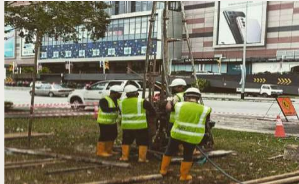
>>> One of the team conducting a standard penetration test at one of the proposed ART station sites near a popular shopping mall on Jalan Wan Alwi, along Blue Line.
